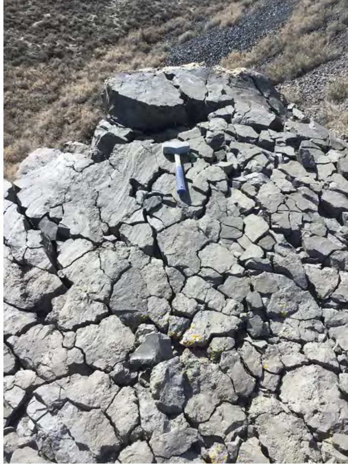
Figure S2.5. The knob of rhyolite that was sampled for cosmogenic exposure dating was in situ and composed of columnar jointed rhyolite. The top 3 cm of rhyolite that was at least 4 cm from an edge was collected and cut for analysis. Hammer for scale.
